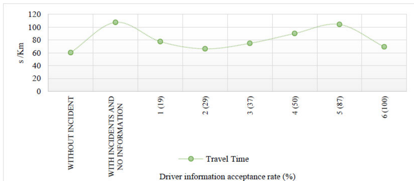
Fig. (25). Travel time across scenarios by user information acceptance rate in the influence area of street 33 and street 48. Source: Authors’ elaboration.
