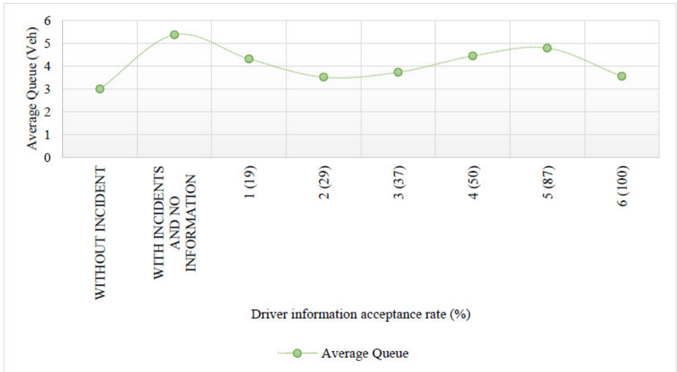
Fig. (24). Variation in average queue length across scenarios according to user information acceptance rates in the influence area of street 33 and street 48. Source: Authors' elaboration.
