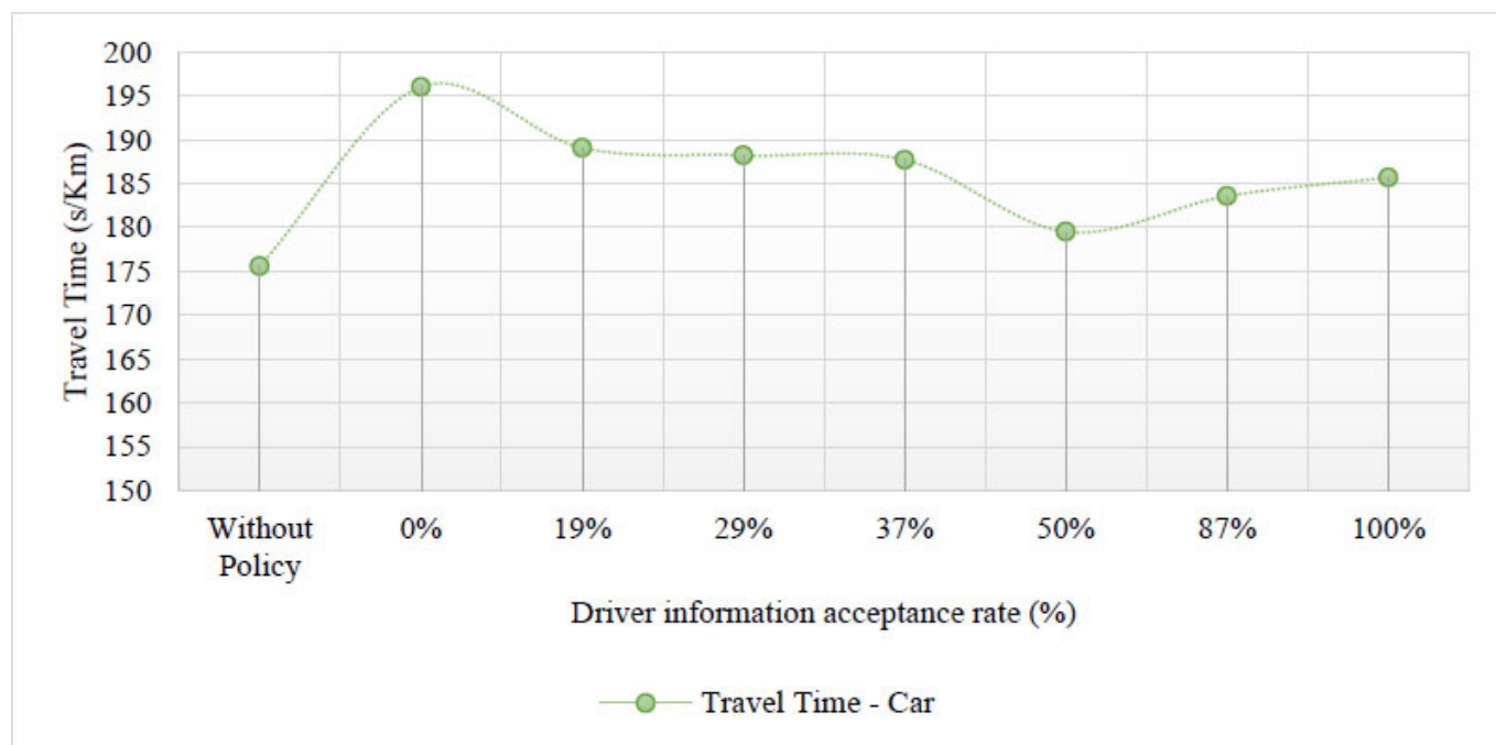
Fig. (21). Travel time by percentage of traffic information accepted by users in Bucaramanga. Source: Authors' elaboration.
