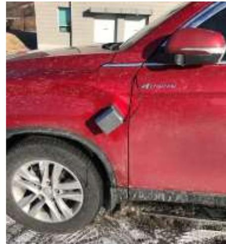
Fig. (2). Surface temperature sensor.
